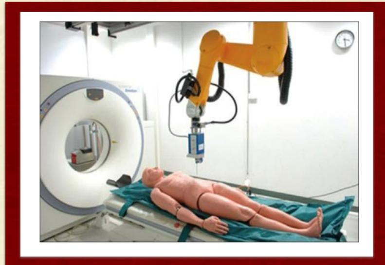
Image #1. An example of a virtibot system with a biopsy module.<sup>4</sup>
